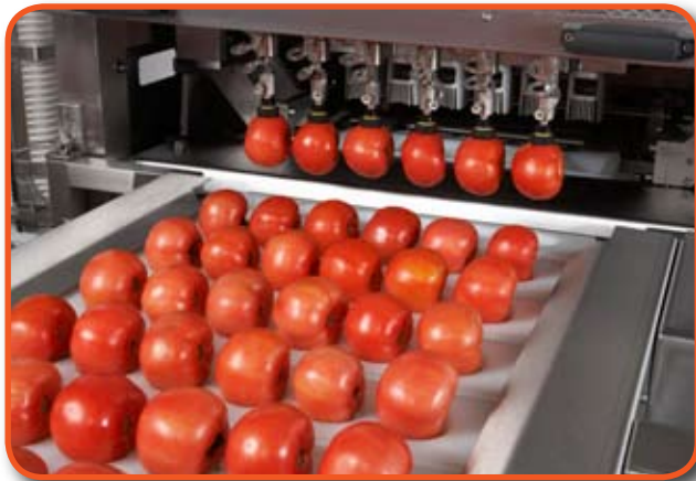
Fully integrated Pick & Place unit, increasing productivity and reducing labor costs.
