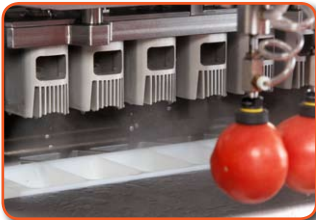
Sanitizes the cutting blades between each slicing cycle, significantly reducing the risk of cross contamination, e.g. In a 10 hour shift the blades will be sanitized over 7,000 times.
