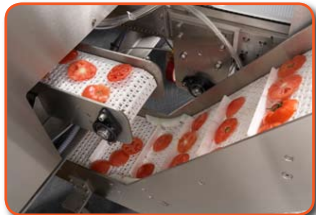
Automatically removes and collects the unwanted end pieces of the tomato.
