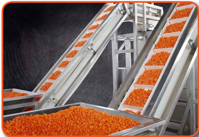
Produce is taken from Hopper by 2 Incline In-feed Conveyors
