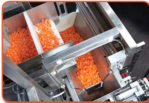
Produce is weighted by 2 precision electronic scales before filling
